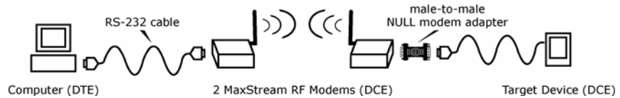
Figure B-02. Example of a MaxStream Radio Modem (DCE Device) connecting to another DCE device
