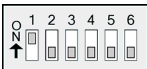
Figure B.8. RS-232 DIP Switch Settings
