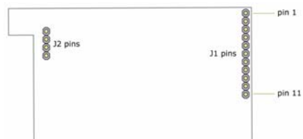
Figure 1.1. XStream OEM RF Module Pin Numbers (bottom view, pins protruding)
