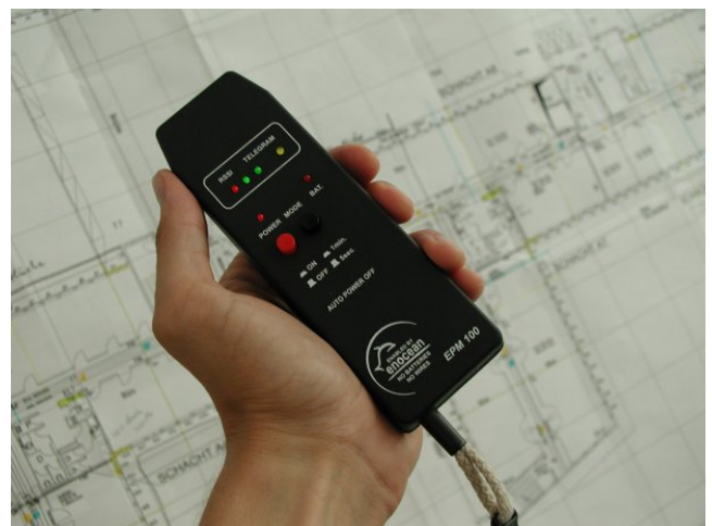
Figure 12: EPM 100 helps to qualify installation positions
